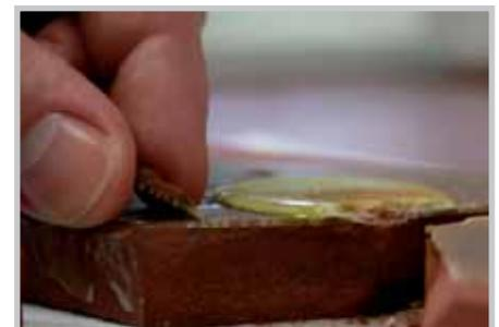
(6) ... the substrate breaks. The quality of the bond is revealed in the detail: After breaking, the primer is still bonded to the substrate. Any potential mechanical damage will therefore not increase.
