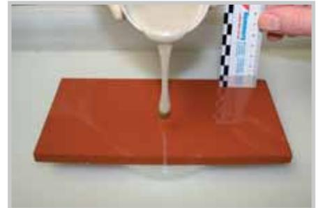
(1) The Remmers Epoxy FAS 100 based primer is poured onto the slab through the water.
