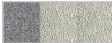
Typically 0.3 mm 0.7 mm 1.2 mm aggregate fractions are used
