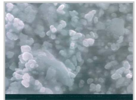
REM photograph of a Bioni coated surface. Here you see the layer close to the surface with nano particles bedded in the binder. (Photograph: Fraunhofer ICT).
